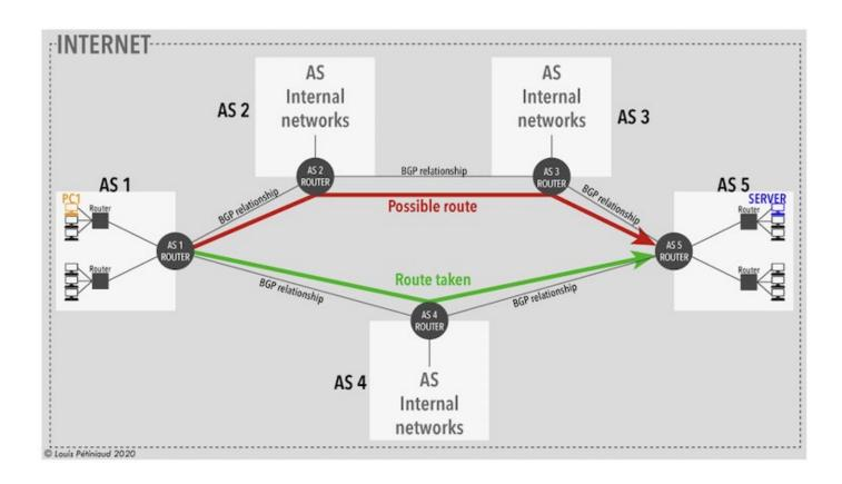
Figure 1: Simplified architecture of interconnections between Autonomous Systems.
