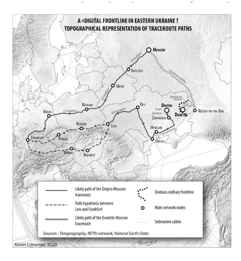
Figure 2: Topographical representation of traceroutes.
