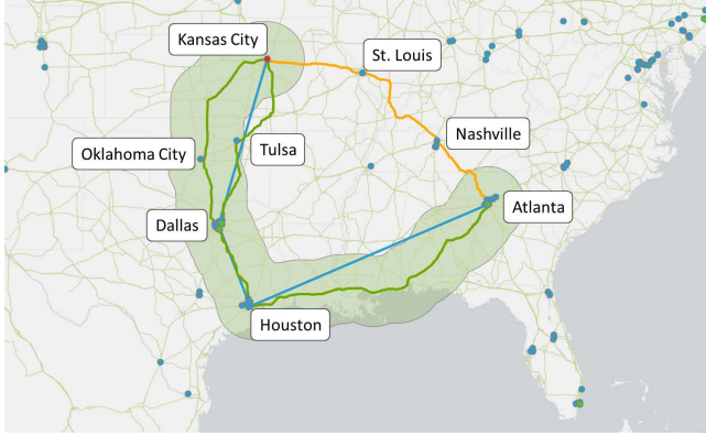
Figure 7: Kansas City to Atlanta traceroute path (blue), inferred physical path through Tulsa, OK or Oklahoma City, OK (green), and shortest practical physical path (orange). AS metro locations depicted as circles with: AS174 (blue), AS12186 (red), AS20473 (green), and AS64199 (purple).
